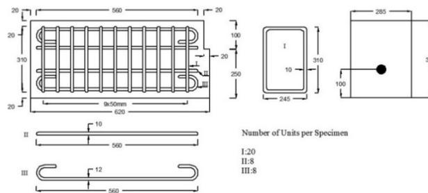
Fig. 2 Flexural pull-out test specimens
