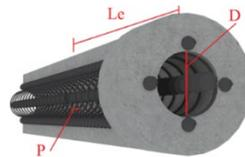
Fig. 1 Details of grouted spirally splice connection
