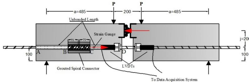
Fig. 3 Flexural pull-out test setup
